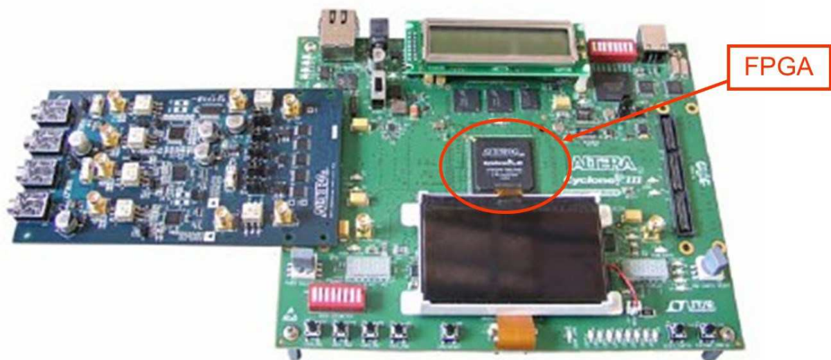
Fig.4. 14 - Board HMSC with stratix III
