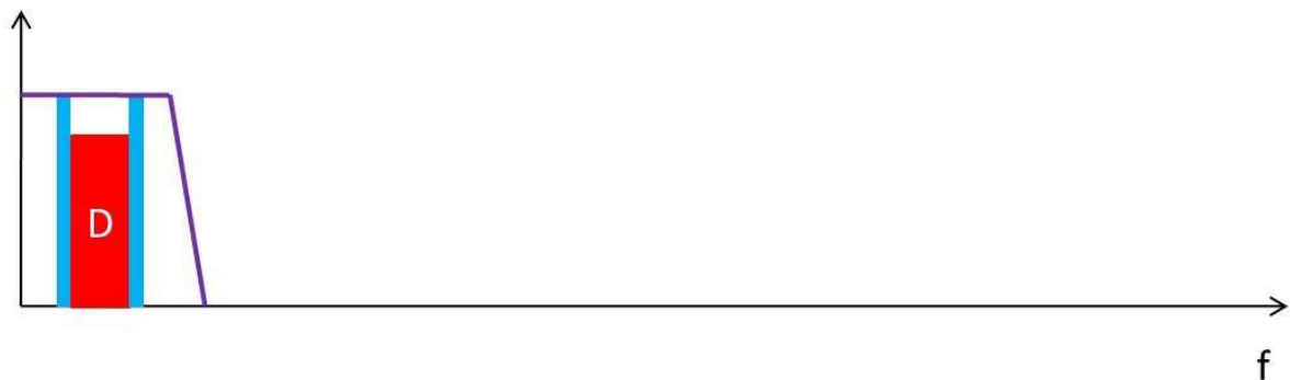
Fig.1. 13 - Wanted channel after mixing and LPF
