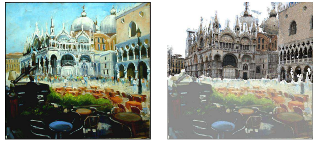
FIGURE 1 – Our system automatically recovers the viewpoint of paintings, drawings, and historical photographs by aligning the input painting (left) with the 3D model (right).
