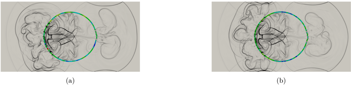
Fig. 4.12: Density field in the fluid and normal stress distribution in the cylinder discretized with (a) 100 particles and (b) 200 particles at time 24.4ms.
