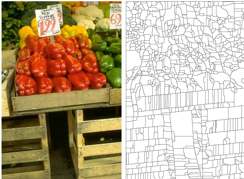
FIGURE 4.5: Initial Image 25098 from Berkeley database, leaves given by lowest (finest partition) threshold of Ultrametric contour map(UCM). The leaves here represents the initial finite net N_0 .
