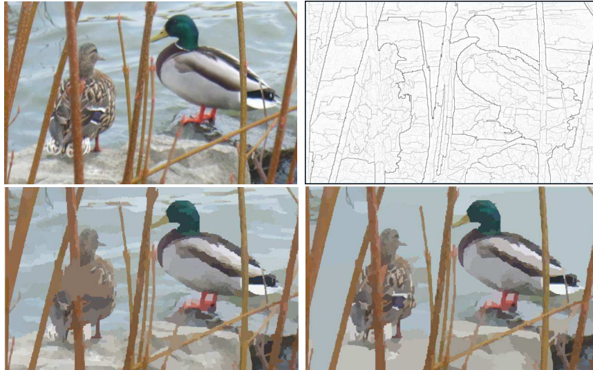
FIGURE 3.1: First row: Initial image and Saliency function corresponding to hierarchical watershed flooding [32]. Second Row: Optimal cuts by using variance of luminance(left), chrominance(right).
