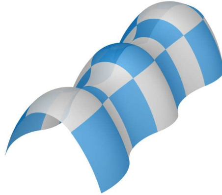
Figure 9: Barrel Vault as a Toric Monge's Surface
