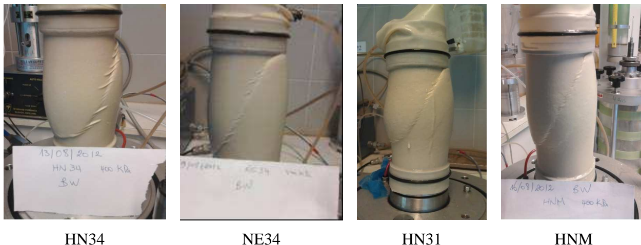
Figure 12- Shear band formation inside the specimens subjected to the horizontal path
