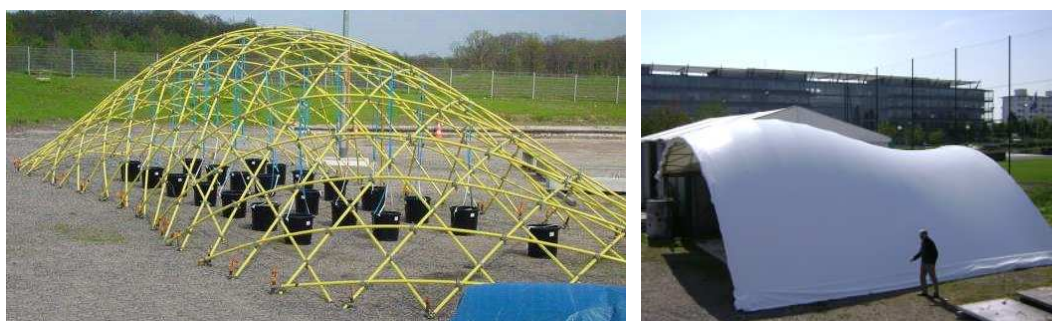
Figure 5: a. First experimental gridshell under testing. b. Second experimental gridshell used as a shelter for a wind tunnel.
