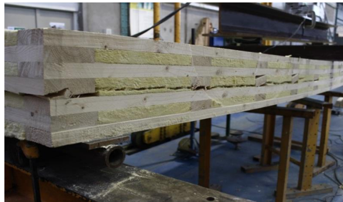
Panobloc ® 1/3, more spaced: rolling shear failure of transverse boards
