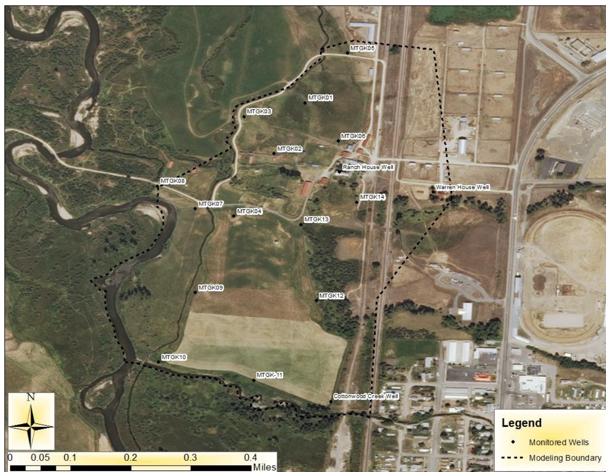
Figure 3. Image of all groundwater wells in the Grant-Kohrs Ranch area. All wells on the figure were sampled except MTGK05, MTGK06, Cottonwood Creek Well, Ranch House Well, and Warren House Well. .
