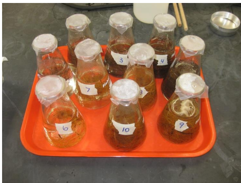
Figure 9. Adsorbent load and isotherm experimental setup
