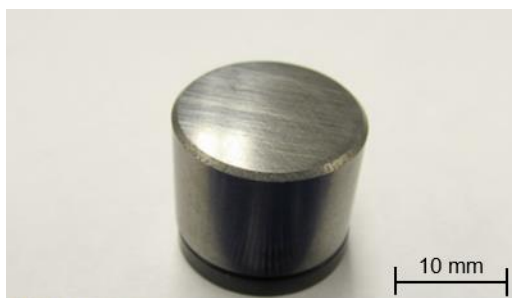
Figure 10. Brazing test sample prior to thermal cycling.
