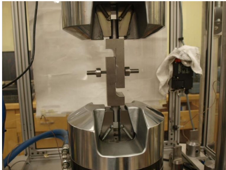
Figure 15. The shear test configuration.
