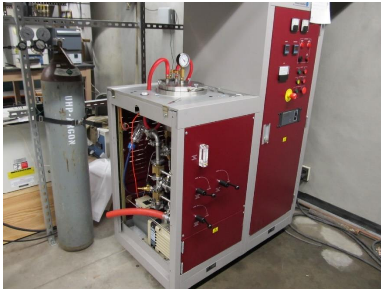
Figure 5. Centorr series LF vacuum furnace.
