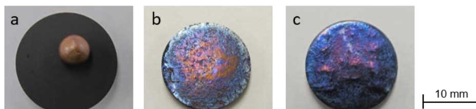
Figure 33. Diamond sessile test samples for silver-copper eutectic-based alloys: a) Ag-Cu with no active metal addition, b) 2 wt% Ti addition, c) 5 wt% Ti addition.
