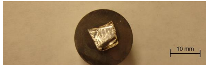
Figure 4. WC-Co sessile drop sample prior to thermal cycle.
