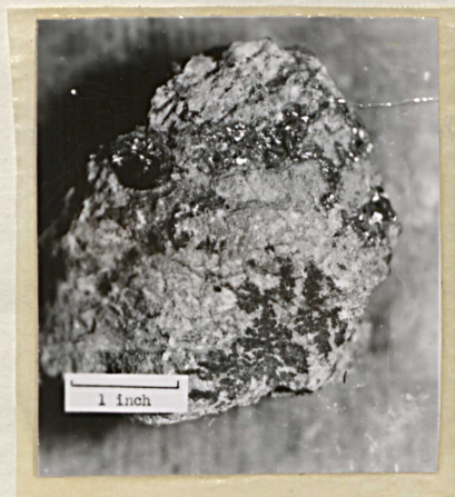
C) Hand specimen showing Dolomite with Galena in upper part and manganese dendrites in lower part. 1/3 natural size.
