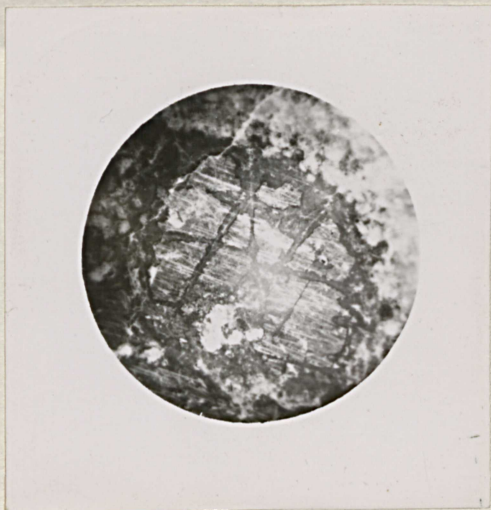
A) Photomicrograph of polished section showing encroachment of Cerrusite on Galena X20.
