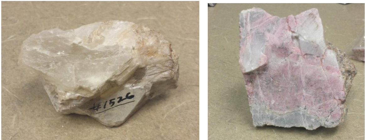
Figure 4: Example specimens of calcite (left) and rhodochrosite (right). Both specimens are about two inches across.
