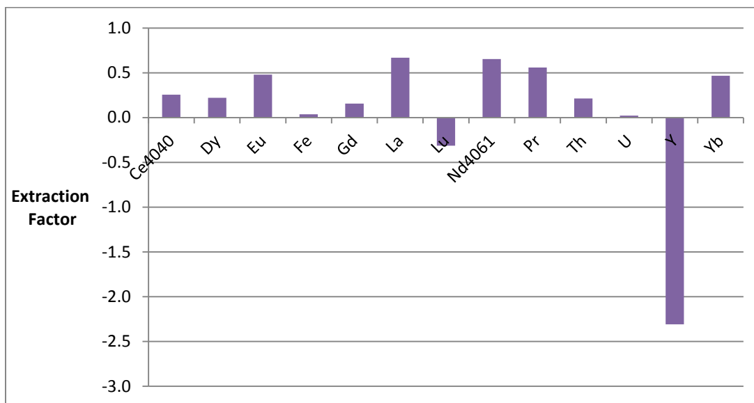
Figure 21: RE4- REE Extraction (0.2g HCl, 90°C)
