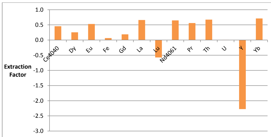
Figure 20: RE4- REE Extraction (5.1g HCl, 60°C)
