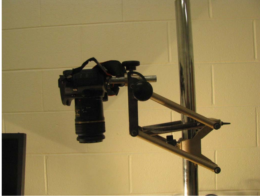
Figure 8: Camera mounting bracket on camera stand
