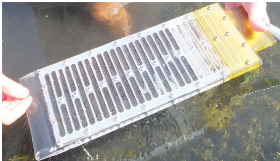
Figure 6. Modified Hesslein diffusion sampler ("peeper").
