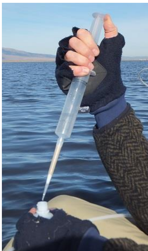
E12. Arsenic speciation performed in the field with a cartridge, with aluminosilicate resin, placed on the end of a syringe. 11/8/2014
