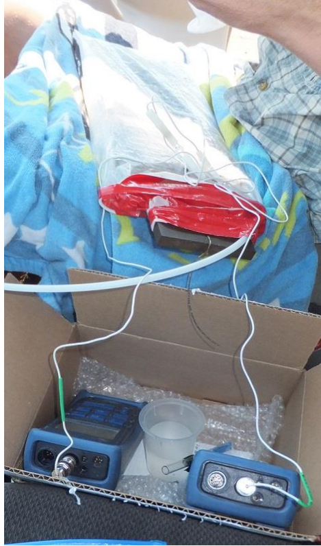
E7. Mini-probes for pH and ORP inserted into Peeper A through glove bag. 8/5/14
