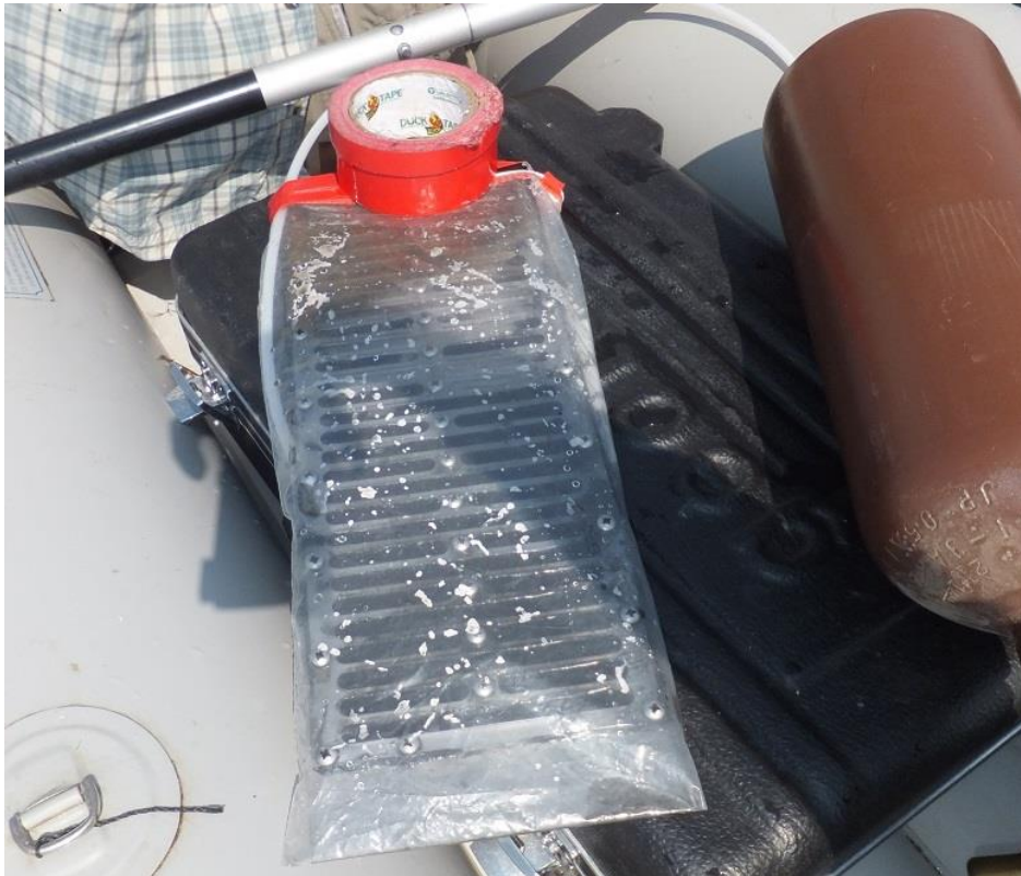
E6. Peeper A in glove bag with argon gas continuously flowing. 8/5/2014
