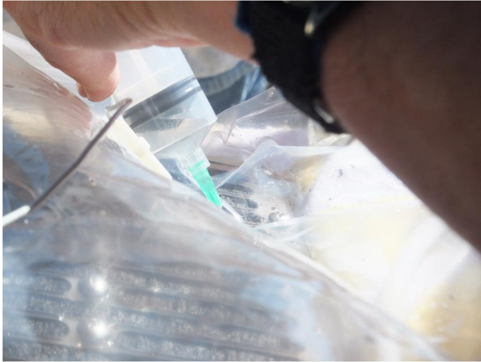
E9. Collecting samples with a syringe needle from Peeper B through the glove bag. 8/14/2014
