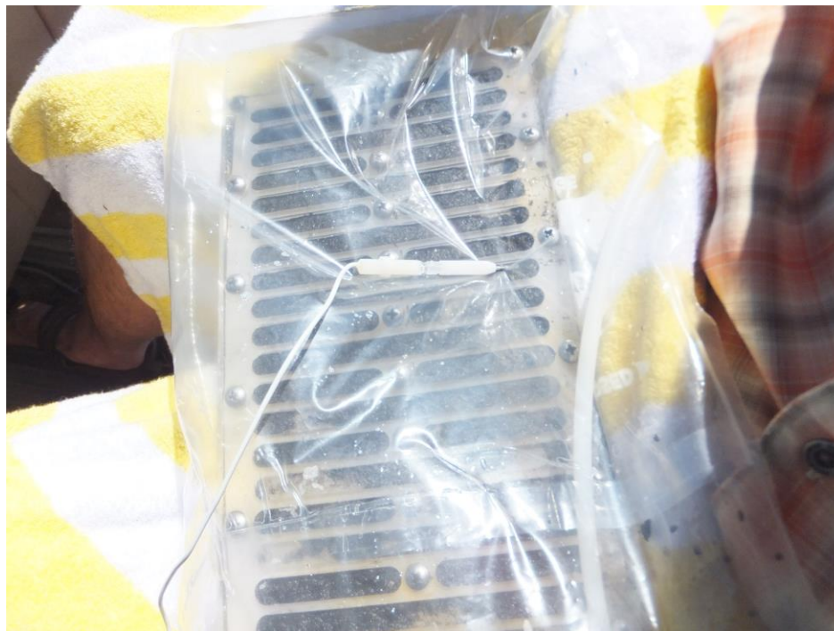
E11. Mini-probe inserted into Peeper B through glove bag. 8/14/2014
