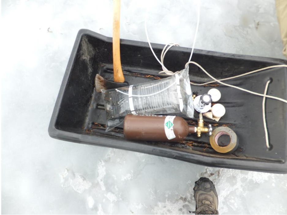
E15. Peeper C in glove bag with argon continuously flowing. 12/6/2014
