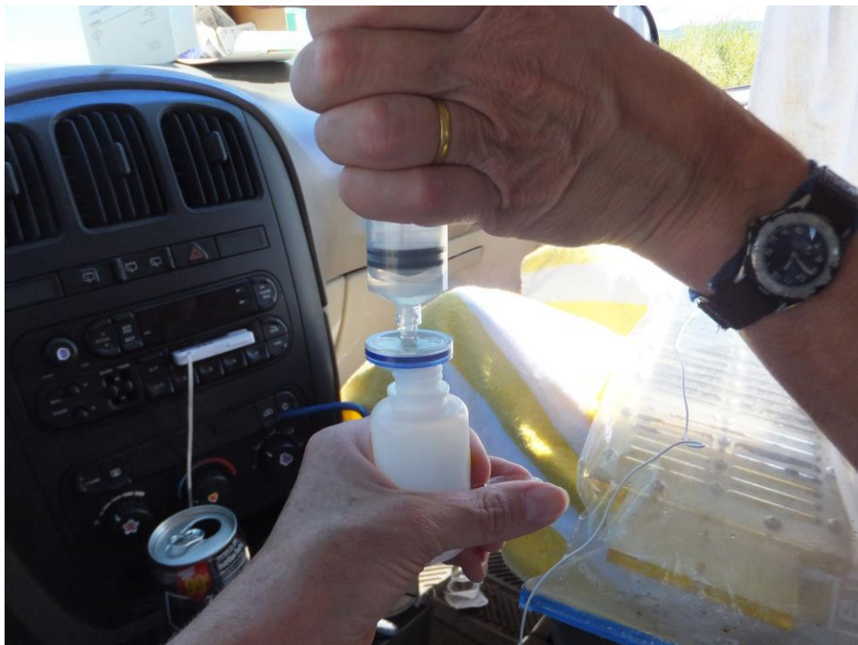
E10. Filtering water samplings into prepared sample bottles from Peeper B. 8/14/2014
