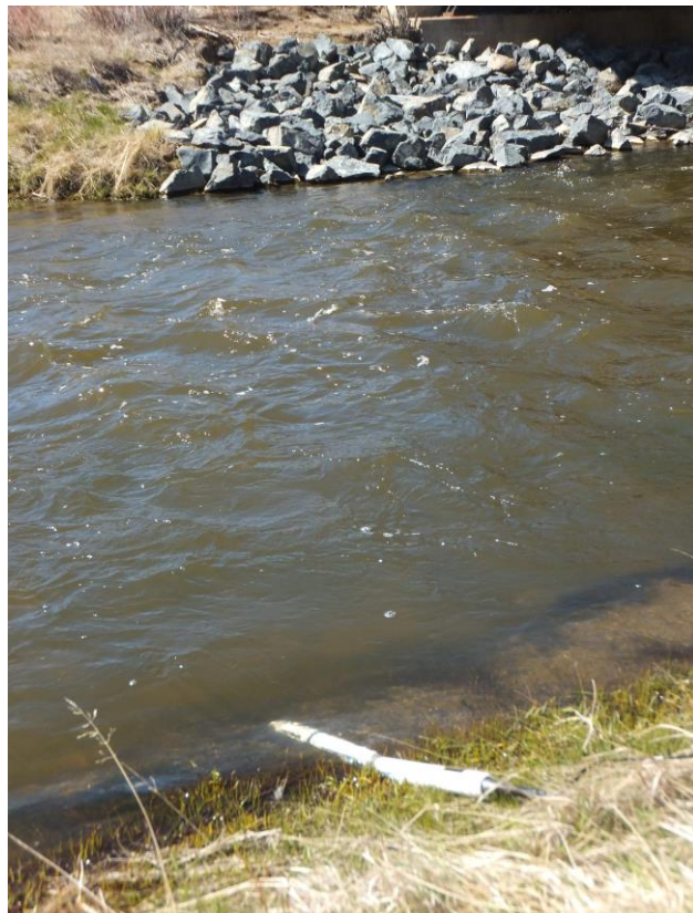
E2. Hydrolab MS-5 collecting field measurements in SBC near the inlet to WSPOU. 5/18/2014
