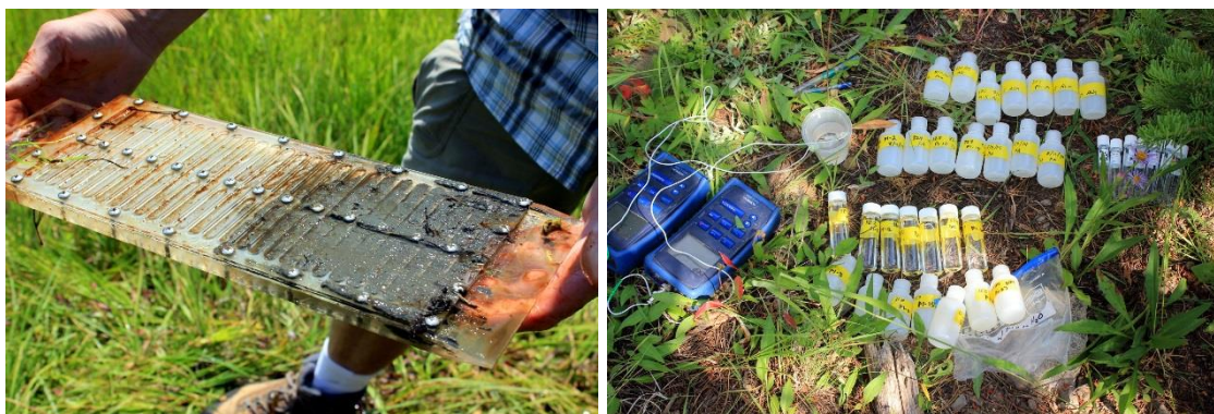
Figure 5: Peeper following collection period & sample suite
