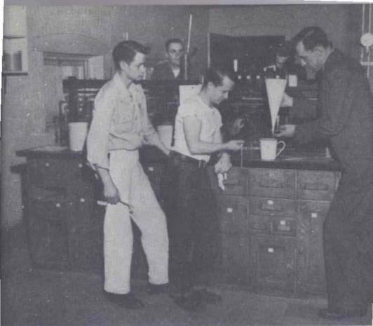
▲ THESE PETROLEUM ENGINEERING STUDENTS are receiving instruction in the use of funnel to measure the viscosity of oil-well drilling mud.
