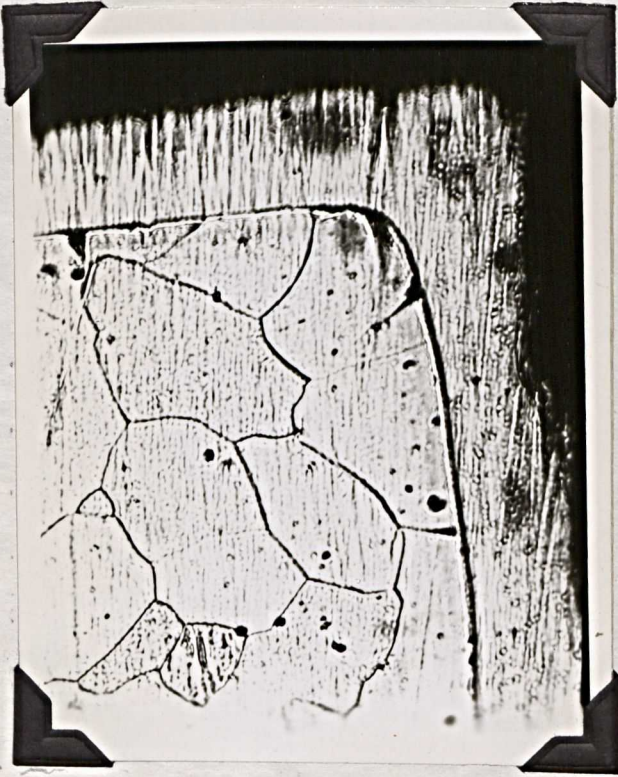
Illustration 2 -- Shows a chromized layer produced on armco ingot iron after two hours at 1850° F. The ferrite was etched 5 per cent picral. Magnification, 200X.
