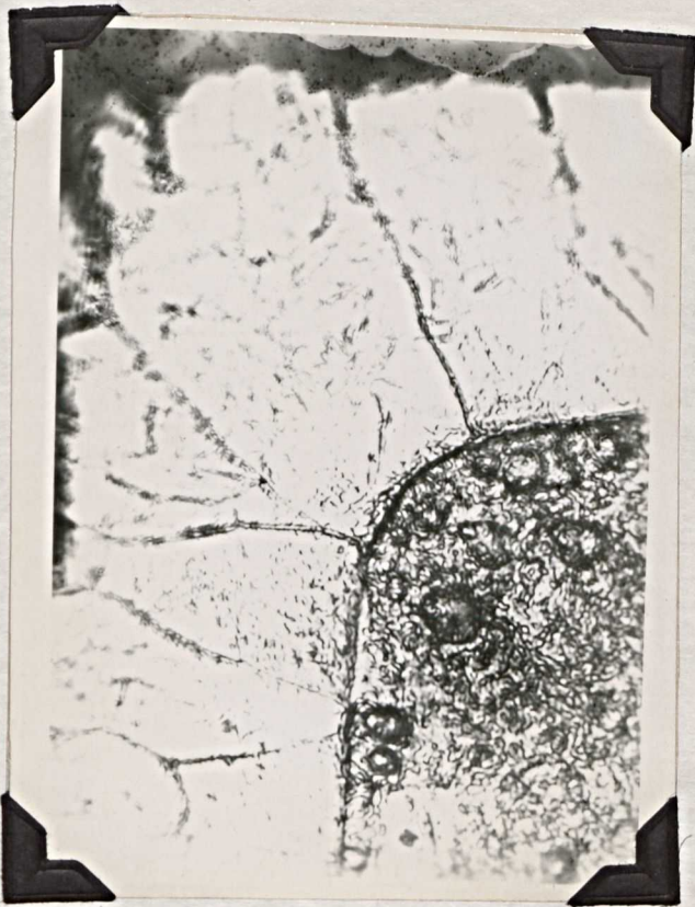
Illustration 4 -- Shows the columnar structure of the chromium layer 200X. The etch used was 8 parts of \text{HNO}_3 , 3 parts \text{HCl} , and 0.5 grams of \text{CuCl}_2 . The etch solution corroded the ferrite grains beyond recognition.
