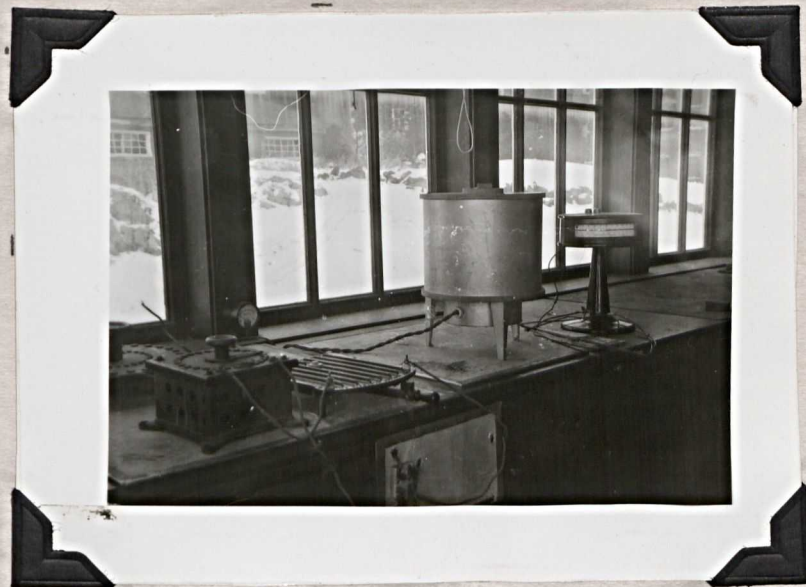
The Sintering Furnace with Thermocouple Plate 3
