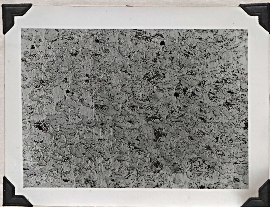
45% Iron, 55% Copper Sintered Compact 100 X, Unetched Plate 6
