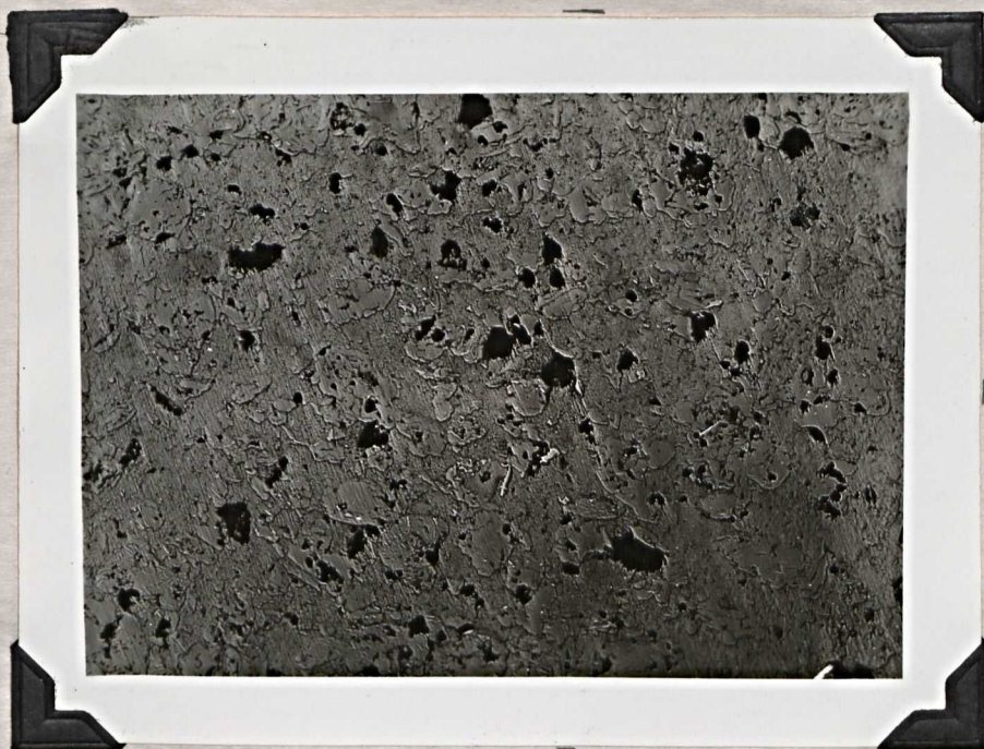
45% Iron, 55% Copper Unsintered Compact 100 X, Unetched Plate 5
