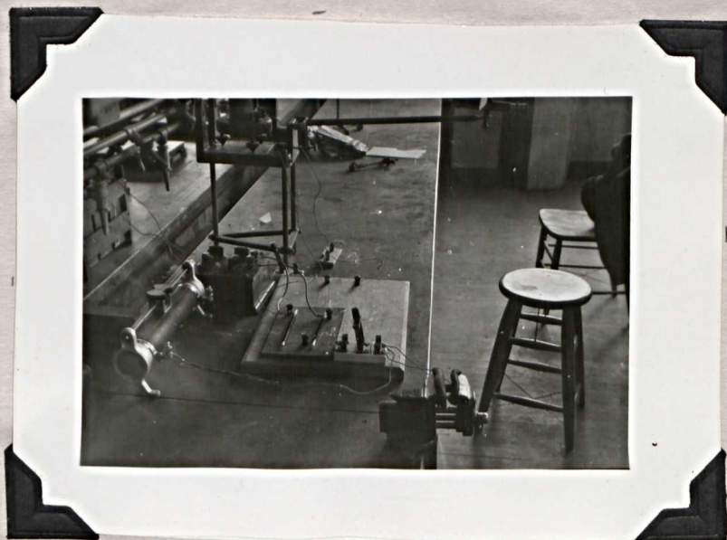
The Electrical Resistivity Measuring Apparatus Plate 4
