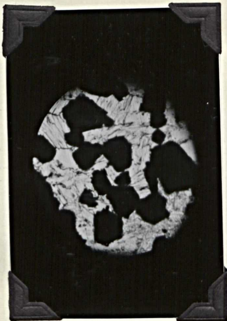
A. Enhedral chromite crystals surrounded by enstatite which is partly altered to antigorite. Ordinary light x 25
