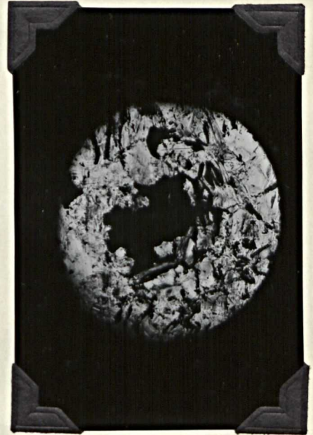
F. Chromite cut by serpentine and antigorite. Ordinary light x 25
