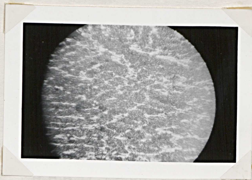
Fig. 7 Pb - 10%Sn, cold-rolled, etched with \text{AgNO}_3 . 100x
