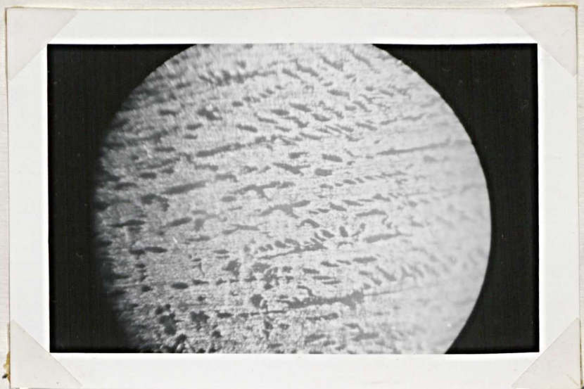
Fig. 5 Pb - 10%Sb - 1%Te, cold-rolled, etched with acetic acid - H_2O_2 . 100x
