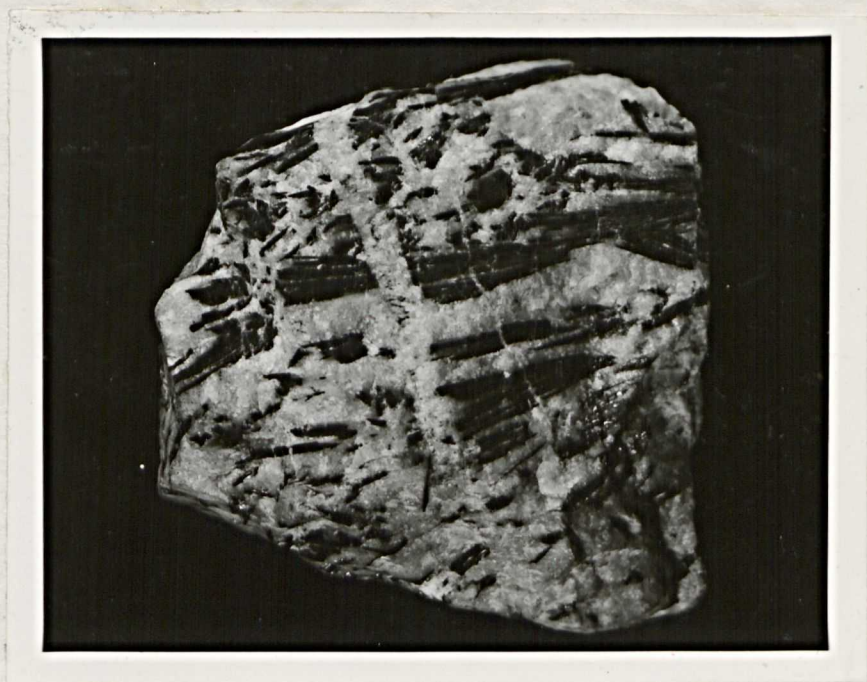
A. Potosi specimen showing broken and displaced hubnerite crystals in quartz. x 4/5
