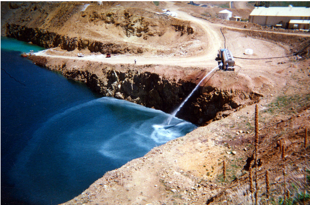
Figure 27. Addition of methanol to the Anchor Hill pit lake. (Photo by Brian Park, May, 2001).
