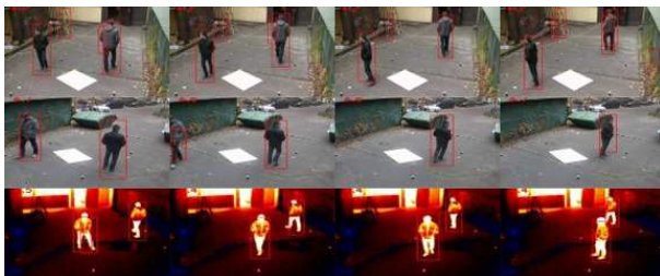
Figure 6. Frames of three different cameras and the detection results (the third camera was an infra one).
