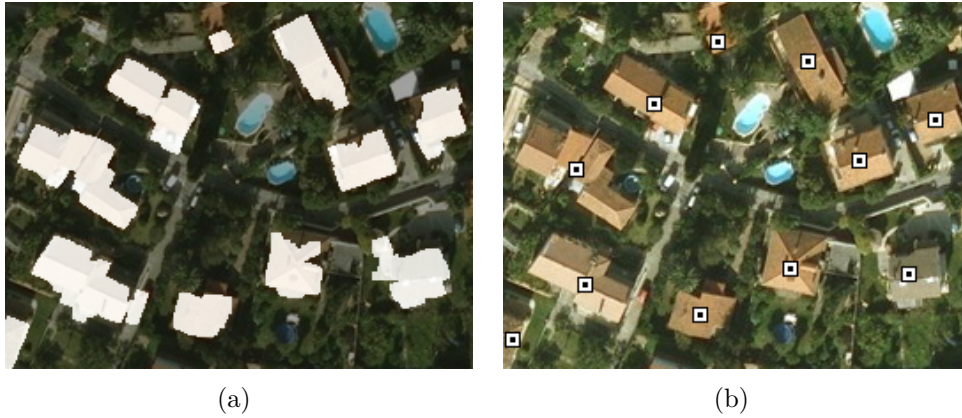
Figure 11: Result of the building detection: (a) shows the detected contours; (b) defines the estimated locations of the detected buildings.
