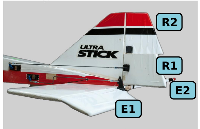
Fig. 2. Tail of the FASER UAV with the control surfaces labeled (E – elevator, R – rudder).
