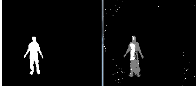
Fig. 2: The image on the right was made with the in-built motion detector class of the OpenCV. We can see, that the motion mask is not perfect, and the image contains noisy pixels.
