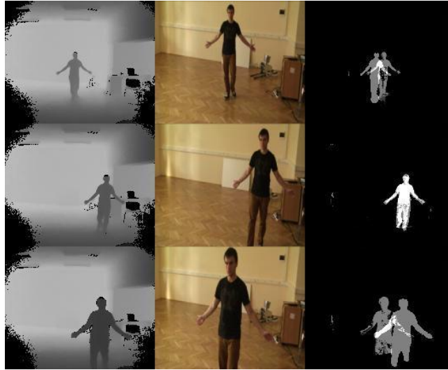
Fig. 3: In these pictures one can see in the first column the outputs of a depth sensor, in the second column the outputs of a conventional camera and in the third column the image after merging the motion masks of these two sensors First row: The object is placed behind the proper plane of the homography Second row: The object is placed in the proper plane of the homography Third row: The object is placed before the proper plane of the homography
