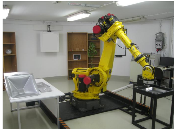
Fig. 6: Set-up for industrial robot-assisted single point incremental forming.
