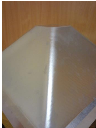
Figure 18 Final part made with SPIF
