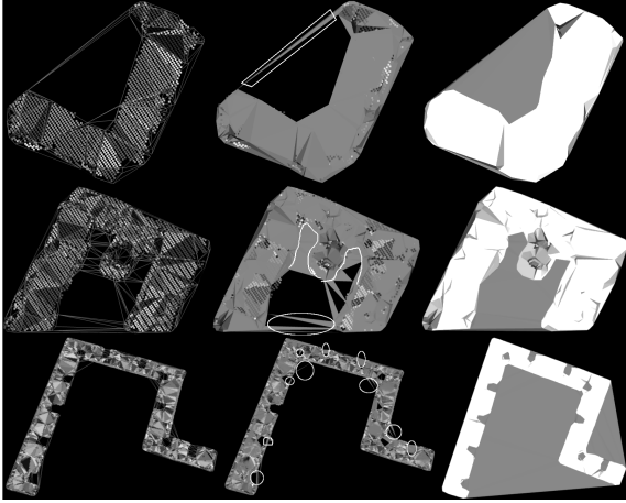
Figure 7: Removing triangles that do not belong to the concave hull. The first two columns demonstrate a hard threshold of the x_s feature, without the MRF smoothing constraint: we can observe several false triangles in the resulting meshes (2nd column). The 3rd column shows the optimal label mask where maximum probability is met. In the first column it can also be observed through coloring how the points are associated to the corresponding triangles.
