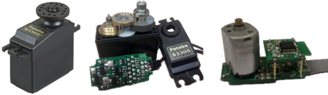
Fig. 1. Futaba S3305 COTS RC servo and the custom servo with measurement and power electronics.
