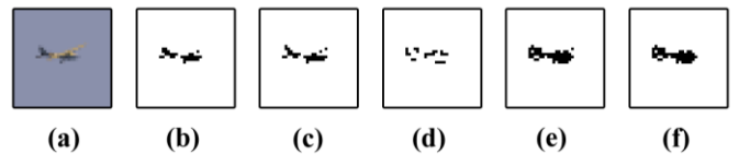
Fig. 11. Segmentation steps; (a) part of the input image, (b) result of adaptive threshold high, (c) result of adaptive threshold darker, (d) result of adaptive threshold brighter, (e) result of closing, (f) segmented image
