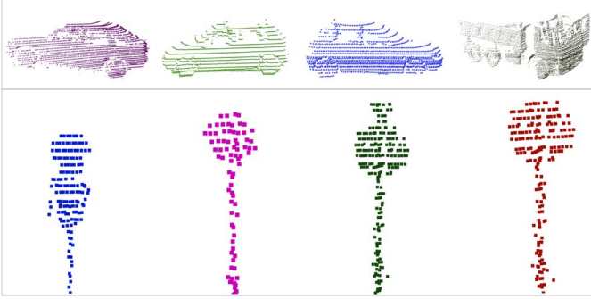
Fig. 8: Qualitative evaluation of the proposed object recognition algorithm. On the top row: Recognized objects with vehicle object class. On the bottom row: Objects which are belong to traffic sign object class.
