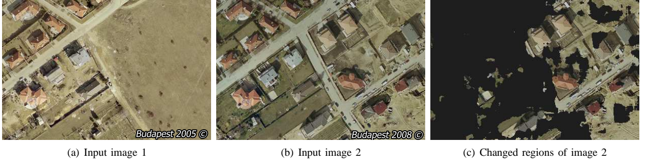
Fig. 6. Low level change detection: (a) and (b) input images, (c) Bhattacharyya change mask \varrho_{ch}
