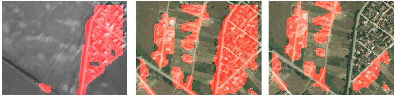
Figure 6. Illustration of the segmentation results after optimization of the proposed MRF model. Left and middle: marking built-in areas in the first and second input images, respectively. Right: marking the built-in changes in the second photo.
