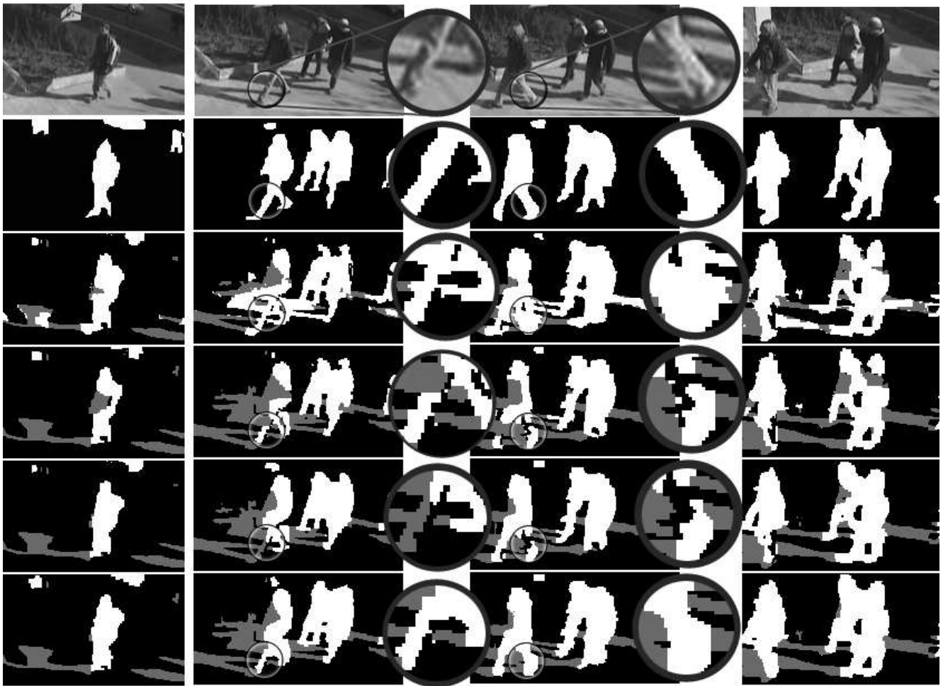
Fig. 14. Validation of all improvements in the segmentation regarding 'Entrance pm' video sequence Row 1. Video frames, Row 2. Ground truth Row 3. Segmentation with the 'constant ratio' shadow model [21], Row 4. Our shadow model with 'uniform foreground' calculus [22] Row 5. The proposed model without microstructural features Row 6. Segmentation results with our final model.
