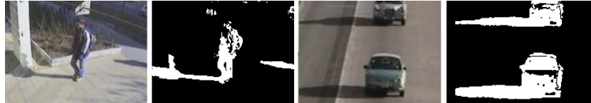
Fig. 1. Results of foreground detection with Stauffer-Grimson algorithm. Left: School Entrance in the afternoon ('SE pm') video, right: 'Highway' test sequence.
