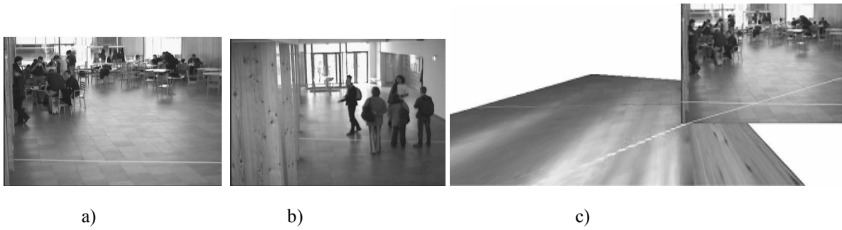
Fig. 8. Images of “Main hall” and “Entrance” cameras with control lines on the ground (marked with two long paper tapes) for verification. Result of alignment of non-overlapping views with the highlighted control lines in c).
