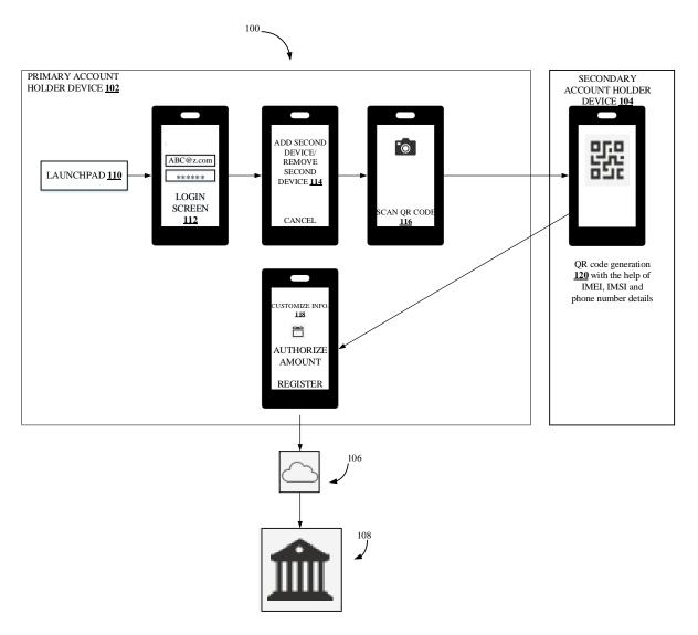
Figure 1: Registration of Secondary account holder device with primary account holder device
