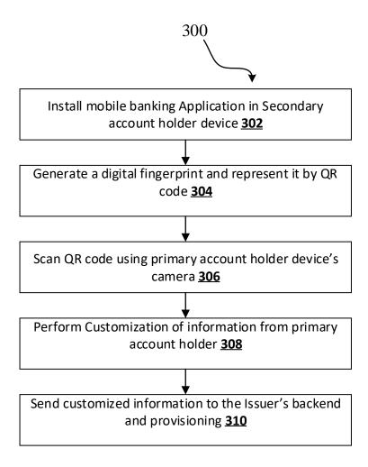
Figure 3: Flowchart for method of Registration of Secondary account holder device
