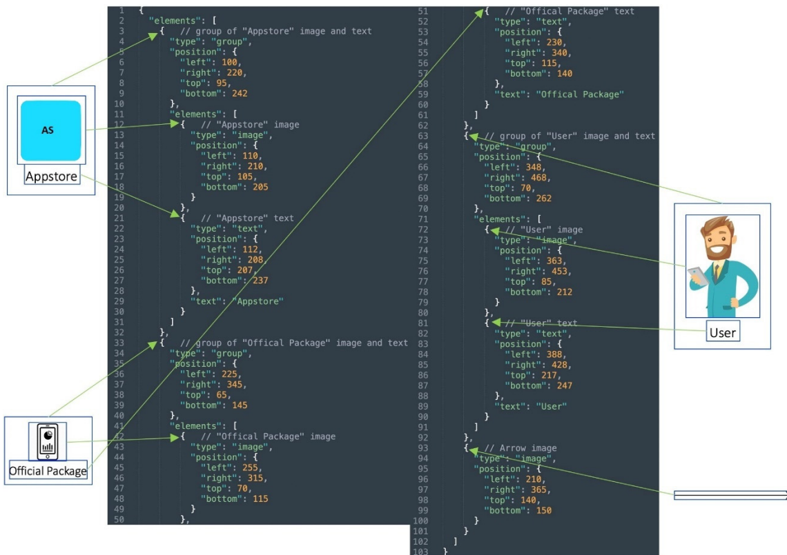
Figure 11B: Step 2 – Reconstructing Hierarchical Structure
