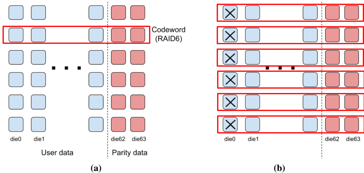
Fig. 2: Codewords in NAND flashes
