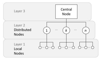
Fig. 3 Laminar control scheme [7]
