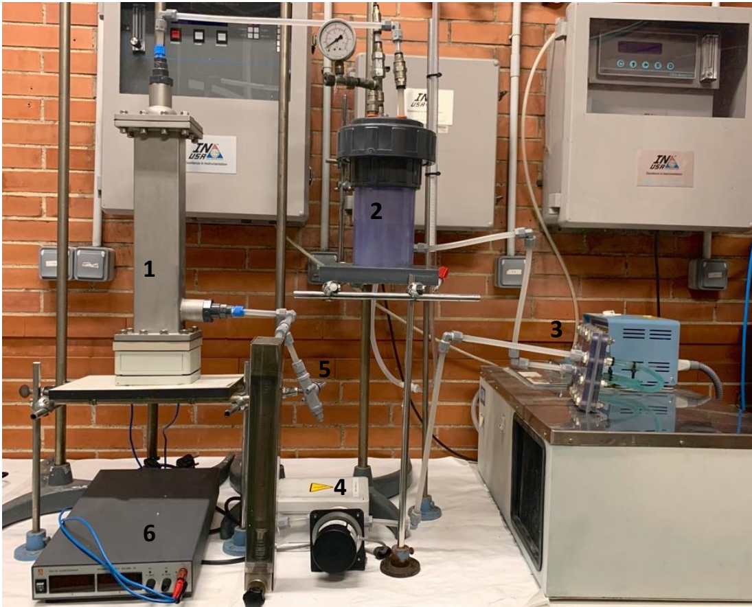
Figure 1. Experimental setup for the discontinuous mode: 1) reactor; 2) tank; 3) heat exchanger; 4) micropump; 5) sampling point; 6) power supply.
