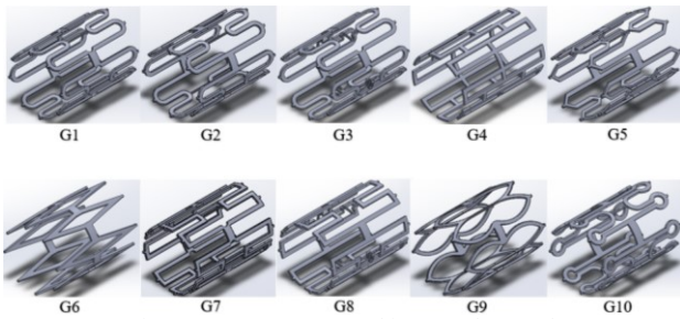
Fig. 7. Stents G1-G10 used in secondary study.
