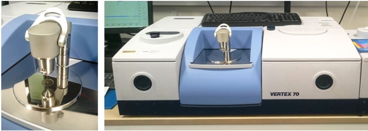
Figure 7: A diamond ATR stage mounted in one of two Bruker Vertex 70 FTIR spectrometers housed at the AMCF.
