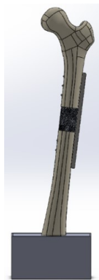
Figure VIII Assembly of the Designed Scaffold and the Fixation Plate
