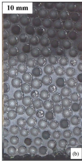
Figure 1. Cell structure of an aluminium-stainless Steel composite metal foam specimen (Vendra & Rabiei, 2007)
