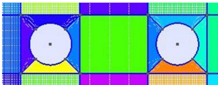
Fig. 5. Enhanced structured mesh around the cylinders
