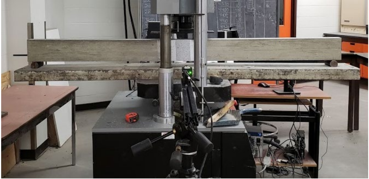
Figure 3.9. DIC system set-up for Batch 2 and Batch 3 beams.
