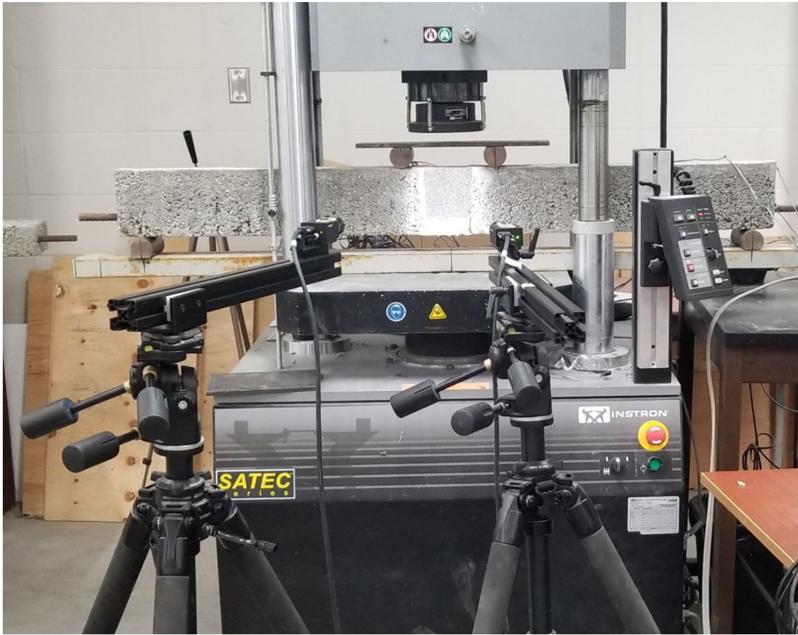
Figure 3.8. DIC system set-up for Batch 1 beams.
