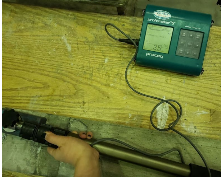
Figure 3.10. Using the Proceq Profometer 5+ to measure the rebar cover depth of a beam.
