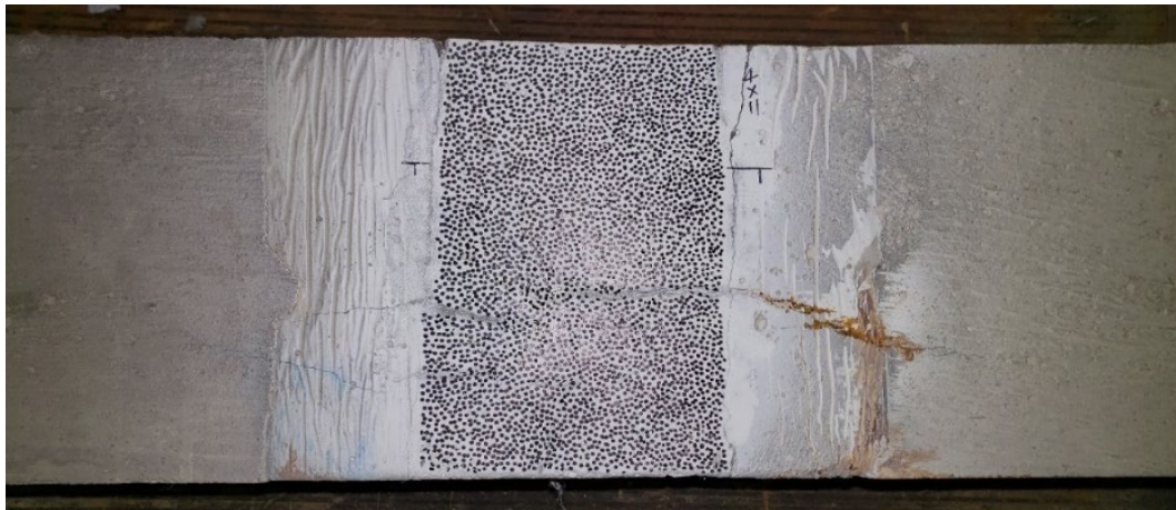
Figure 3.7. Contrasting speckle pattern on the middle section of a beam for the DIC system.
