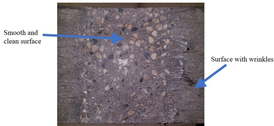
Figure 3.4. A photo of the side surface of a beam from Batch 3 in the middle region, showing wrinkling on the surface and the finish after smoothing and cleaning.
