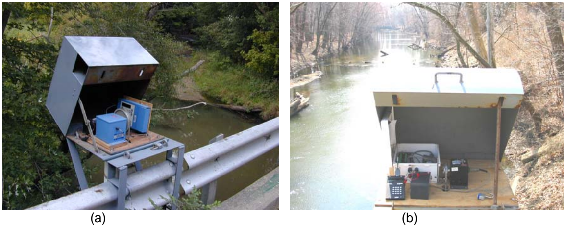
Figure 16. Streamgaging equipment: (a) Leupold & Stevens data logger and (b) CR10X data logger
