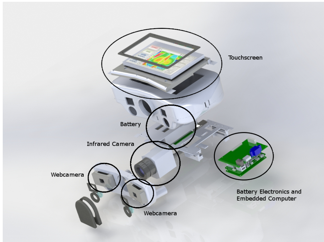
FIGURE 3.4: DFUPS Exploded Plan - One of the web cameras was not useable due to USB bandwidth limitations and was replaced by a speaker
