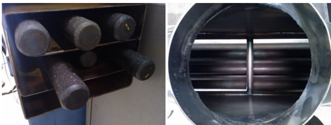
Figure 4-5 – Internal pictures of the heat exchanger
